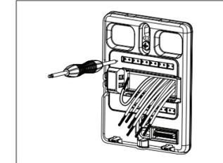
Use terminal release tool to release the spring closure and then insert the wire. (A paper clip or similar tool can be used as an alternative.)
