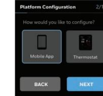
Upon initializing, the thermostat prompts the user to choose the platform for configuration. Follow the prompts, either in the Mobile App, or thermostat display, to complete the set up and basic configuration.
